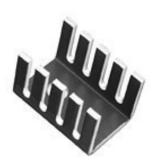
Cross Reference: 6078B Height: 9.65mm Mount Orientation: Vertical and horizontal Finish: Black Anodize RoHS: Compliant Thermal Resistance: 25.9℃/W
